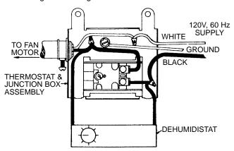
Figure 7 — Wiring Diagram for Dehumidistat
